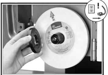
Figure 25. Wheel ready for removal.
